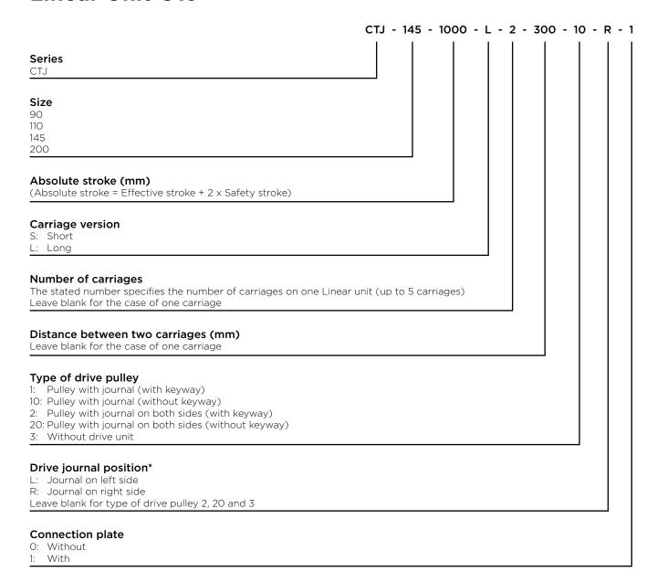
$<sup>^{*}</sup>$  By CTJ 200 with drive pulley 2 or 20, the drive journal position left - L or right - R side must also be specified - motor/gearbox attachment side.
